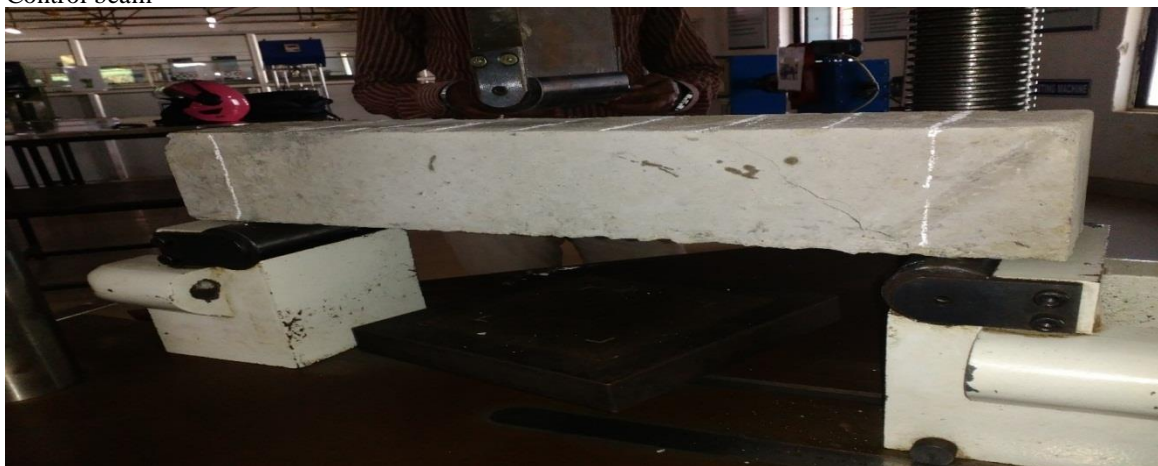
The test result conducted by one point load using UTM Visible Crack
